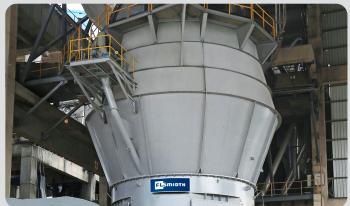
Example of ROKSH separator for optimum cement product quality.
