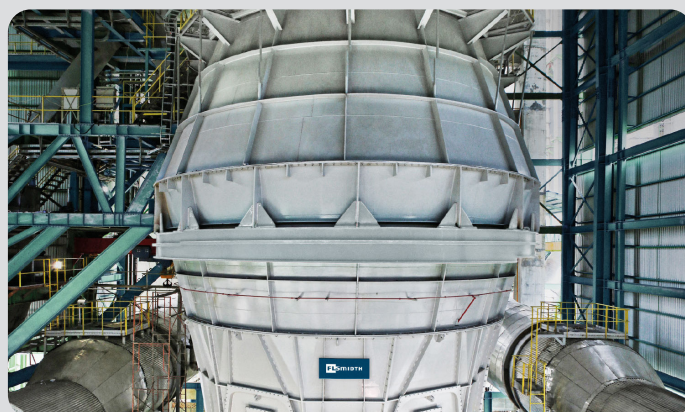
Example of RAR separator for optimum raw meal quality.
